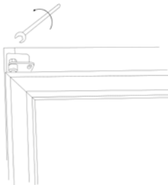
8. Tighten the top hinge pin.
