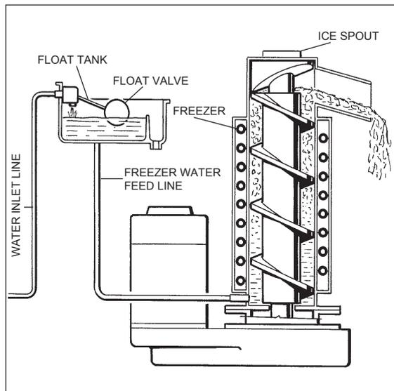
The ice, being constantly lifted up, meets the teeth of the ice breaker which is fitted on the top end of the auger, where it gets compacted, cracked and forced to change from vertical into horizontal motion to be discharged out, through the ice spout and chute, into the storage bin.
