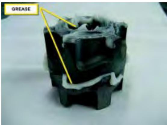
**NOTE.** Install the upper bearing into the ice breaker starting by the radial portion that must be fitted with the flat surface facing up. Apply some lubricant (grease) on the upper surface then install the rollers cage with the smaller openings of the same facing up so to leave a small gap between plastic cage and flat surface of the bottom portion of the bearing (see drawing).
