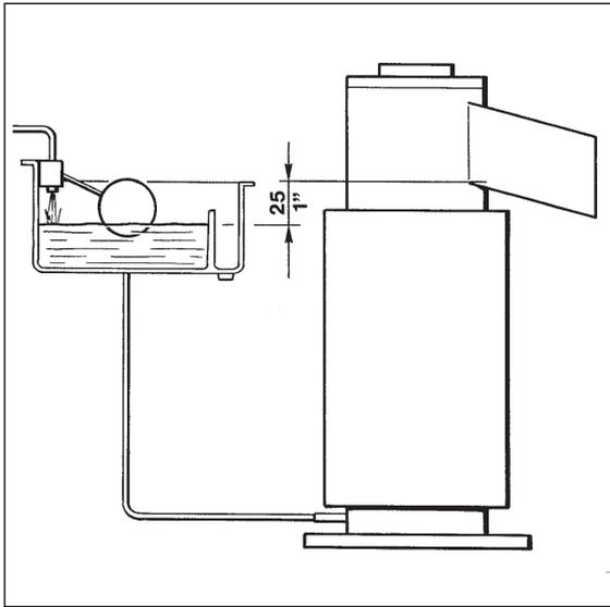
When the water level is above or below the correct one, adjustment can be performed to Raise or Lower the water level by raising or lowering at the measure required, the water reservoir and its mounting bracket.
