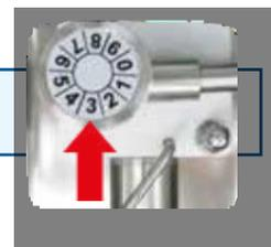
The air valve should be adjusted according to the type of cream used (for example, animal or plant-based cream) and the relative percentage of fat, in order to increase the volume of the dispensed cream as required.
