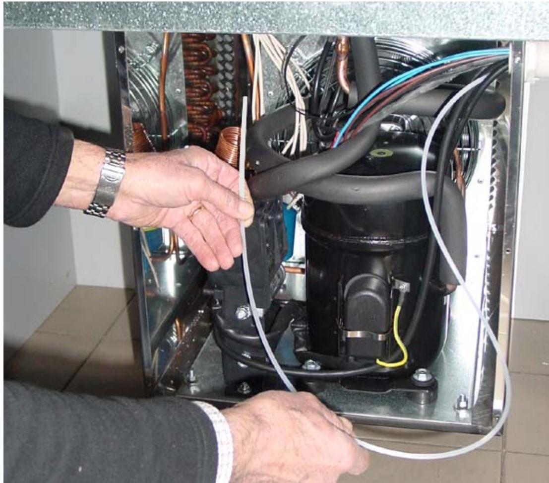
The cable will come out of the large hole drilled in the side 'A'.
