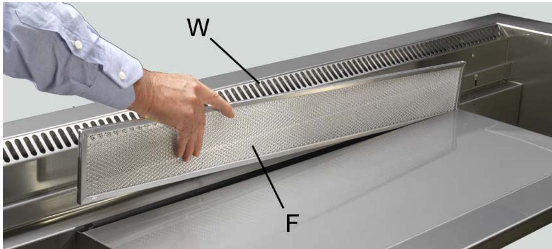
The ventilated models also have an air conveyor 'W' that must be periodically removed and cleaned, which is also useful as it enables cleaning the entire refrigerator unit much better.
