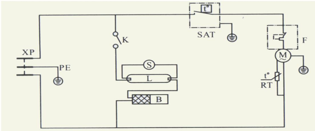
XP-Power supply M-Compressor RT-Startup
