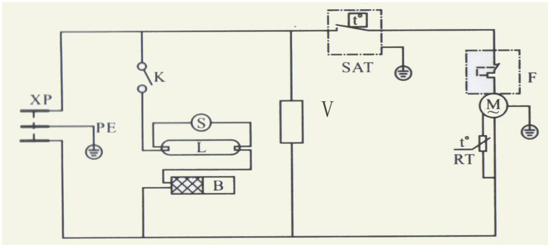
XP-Power supply M-Compressor RT-Startup V-Fan
