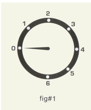
The inner temperature ranges from 0° to 10°. You can turn the thermostat knob to have your desired temperature. Turn the knob clockwise; which the position varies from 1 to 6, you can get a lower temperature inside. Turn the position to 0; you will switch off your appliance. Please see fig #1.
