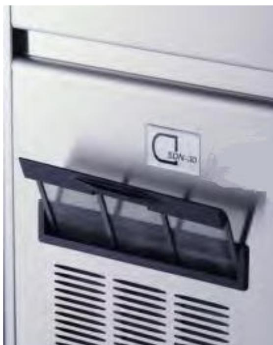
2. Blow pressurised air on the opposite direction of the condenser air flow so to remove the dust accumulated.
