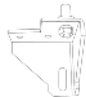
9. Remove the bottom hinge pin and turn the bottom hinge 90 degrees.
