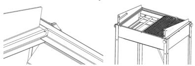
1. First attach the side panels and make sure they are securely fastened in the groove at the front.
