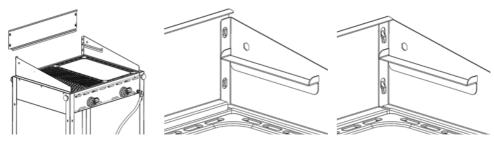
2. Slide the rear panel in position between the side panels.
