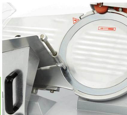
Hardened stainless steel hollow ground blade
