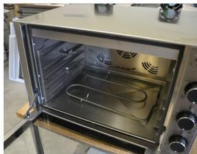
For the assembly, proceed in the reverse order. Take care, place the bottom heating element in the right way
