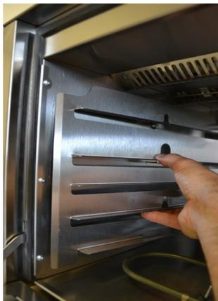
To replace the scales, place them on the 2 pins, press slightly and let slide down.
