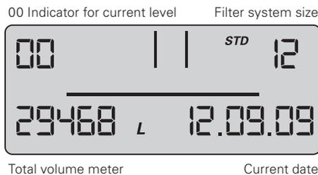
The total volume meter is managed at this level; it counts up from 0 irrespective of the cartridge change.
