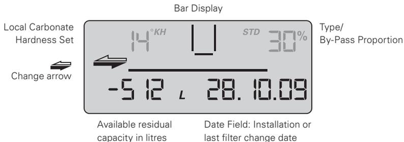
If the monthly limit has been reached up to a month before expiry of the set time limit, it is signalled by the date field flashing.
