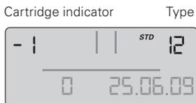
Date of inserting the cartridge
