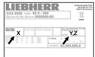
The nameplate shows the Liebherr logo, model 'XXX 9999', and climate class 'X'. It also indicates the temperature class 'Y,Z' and the R600a refrigerant.
