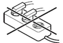
**Connect the appliance with a properly earthed fused plug and socket only.**
